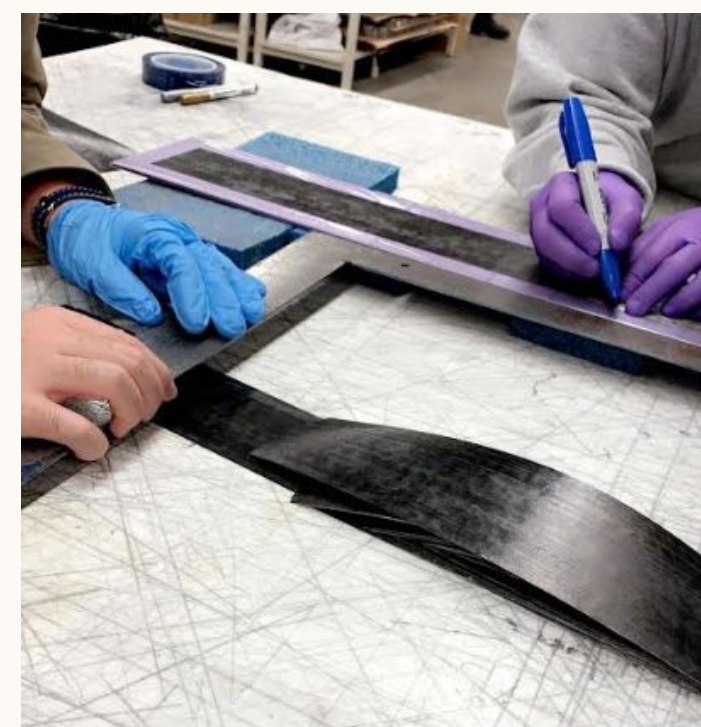
Figure 2: Students organizing and marking up tooling for the beam layup
