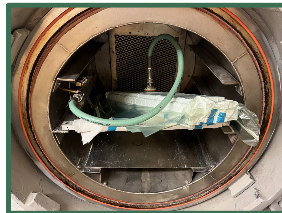
Figure 4 - Beam Layup on Tools in Autoclave
