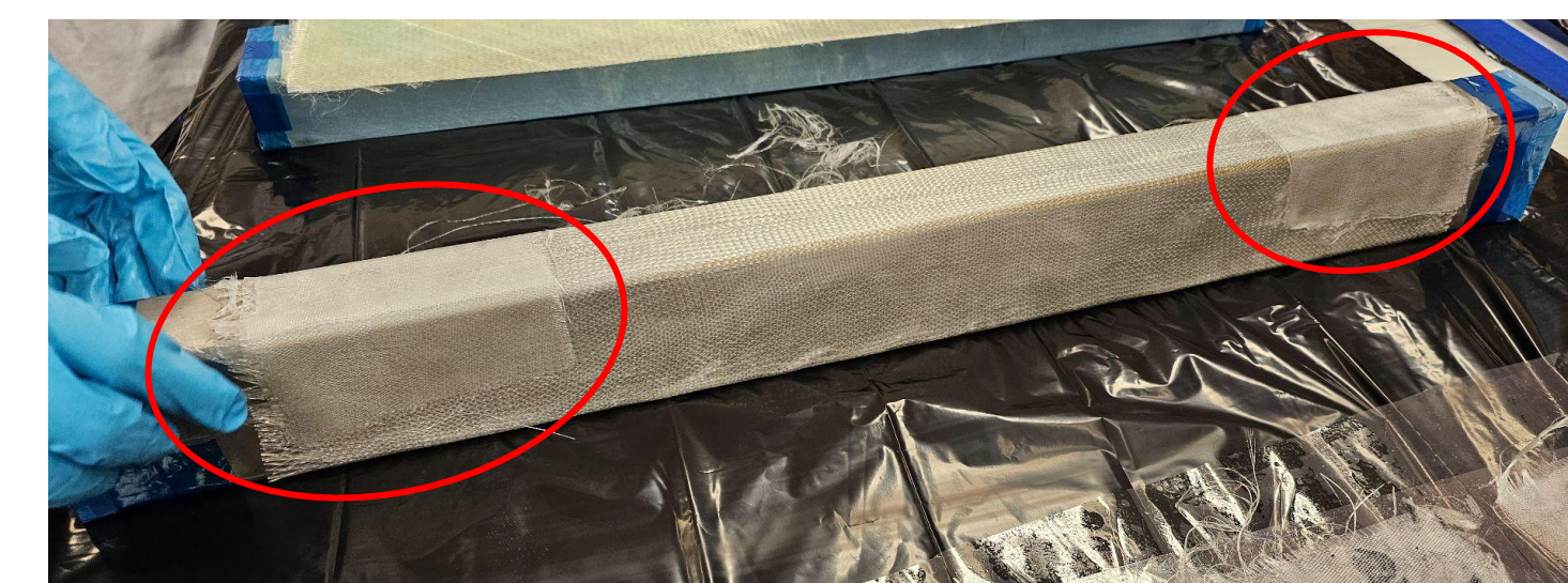
Figure 7: Tabs added to the center web part at the ends, encircling the tool.
