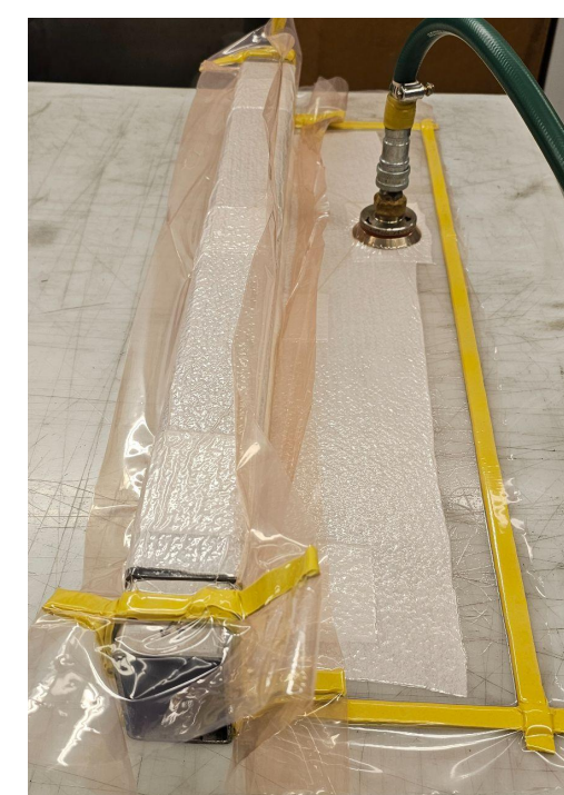
Figure 3: Vacuum-bagged web part for debulking.
