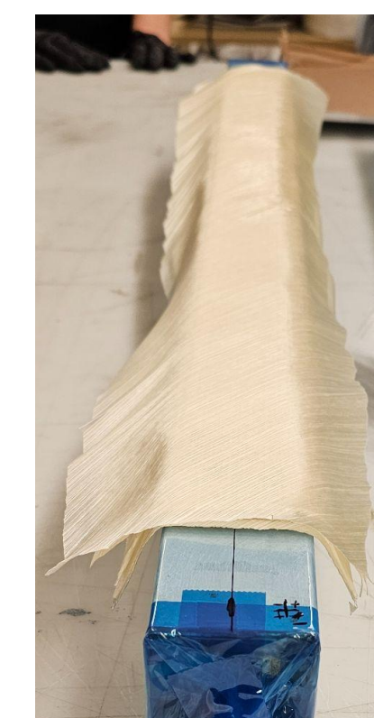
Figure 5: Wrinkage as plies are individually bent around web tooling.
