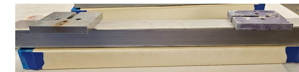
Figure 6: Pressing plies with steel weights.
