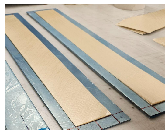
Figure 2: Top and bottom flanges laid up on tools.
