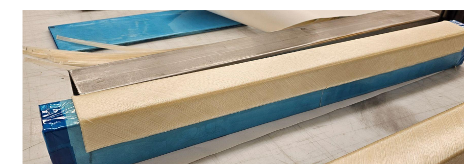
Figure 7: Laid-up web created using new method.
