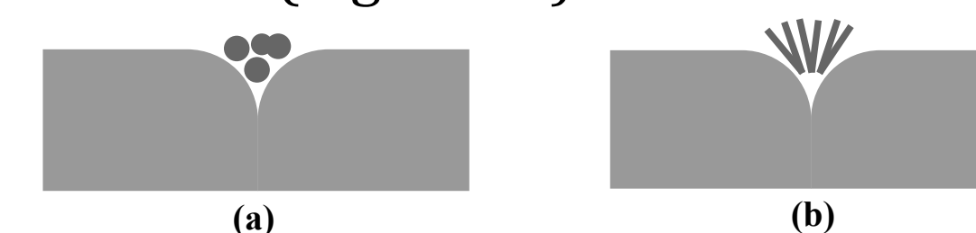
Figure 8: Cross-section diagrams of noodle packing methods. (a) Twisted strips. (b) Folded strips.
