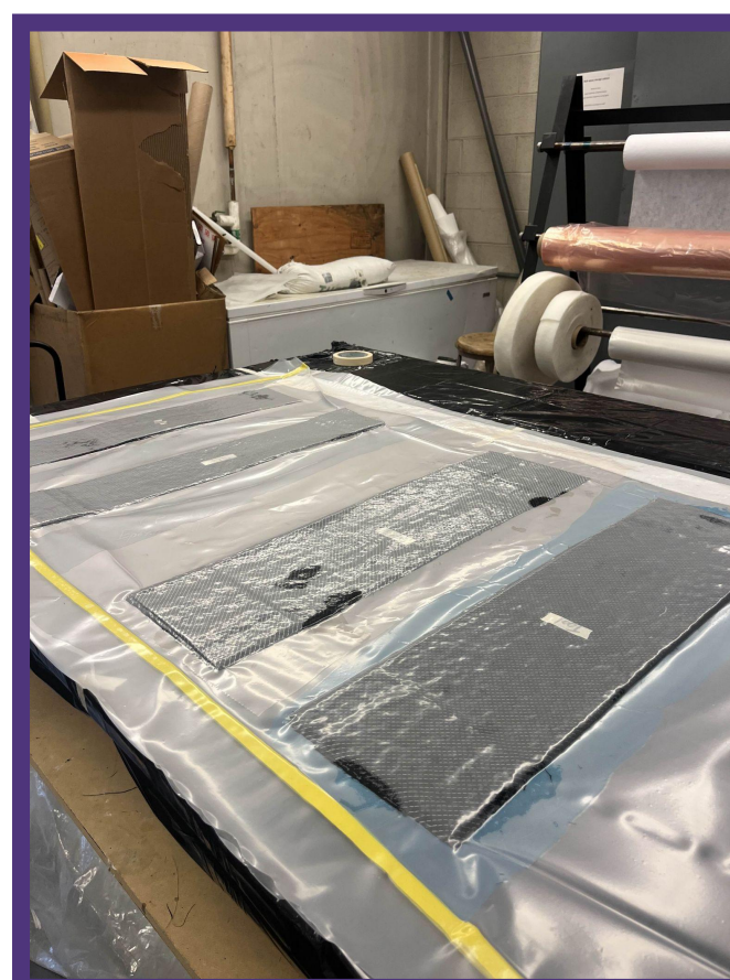
Figure 2. Vacuuming plies and resin to distribute resin evenly
