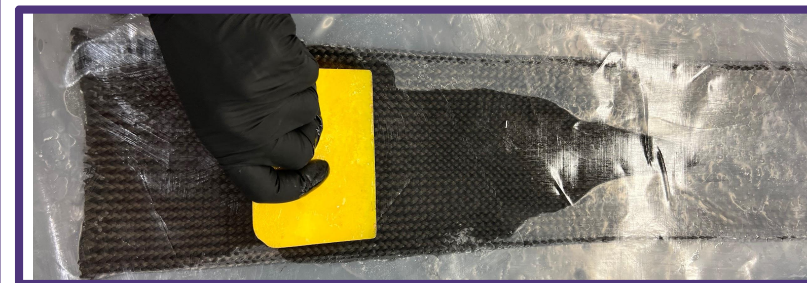
Figure 7: carbon box ply having resin applied.
