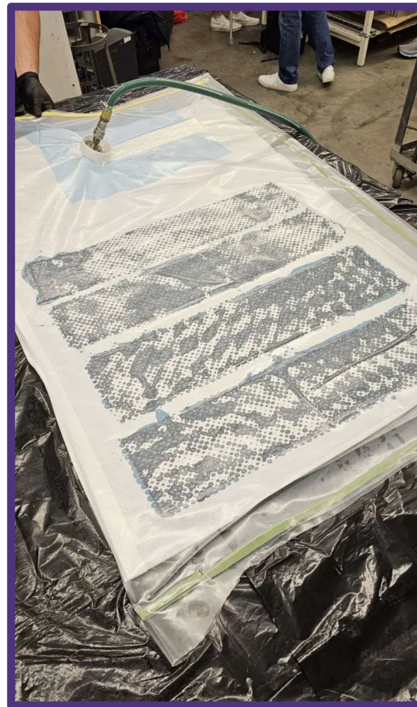
Figure 2: carbon box plies being debulked under vacuum before going on the tool.
