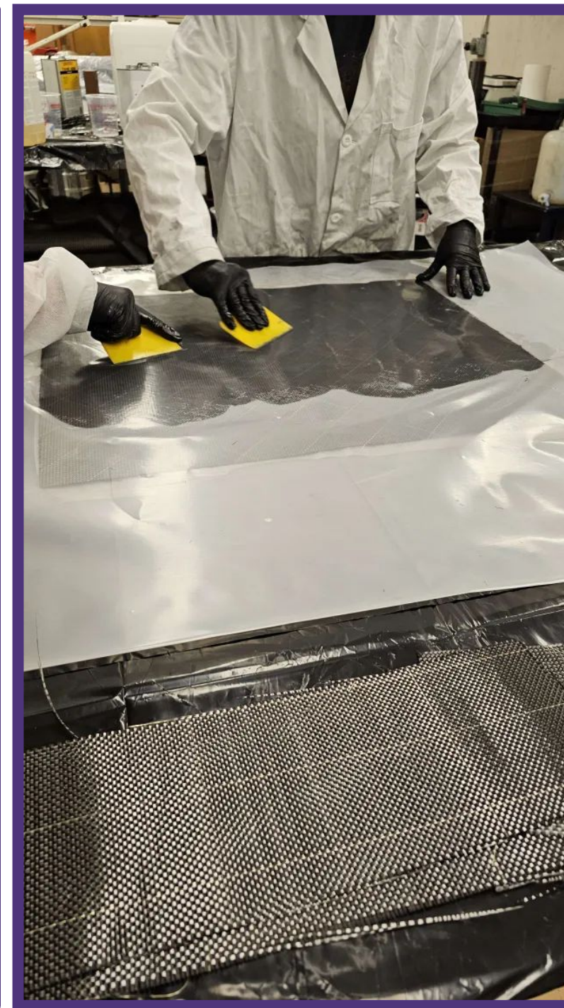
Figure 3: carbon box substitute sock being saturated with resin before application.
