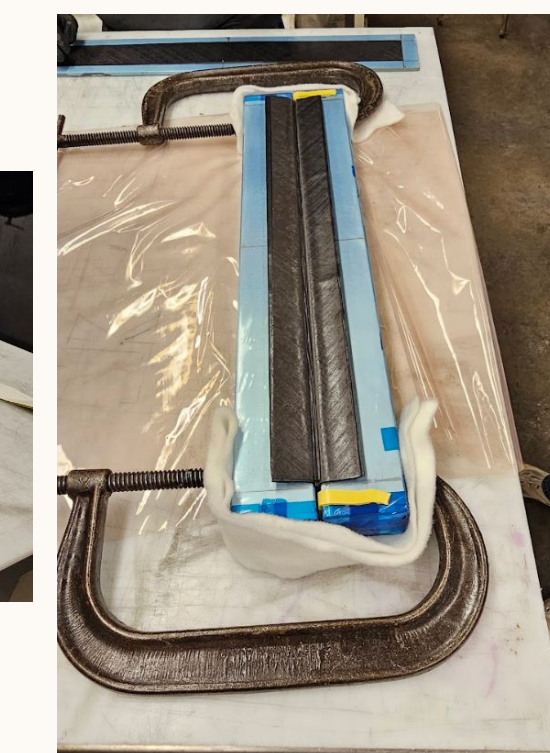
Figure 6: Webs assembled into I shape
