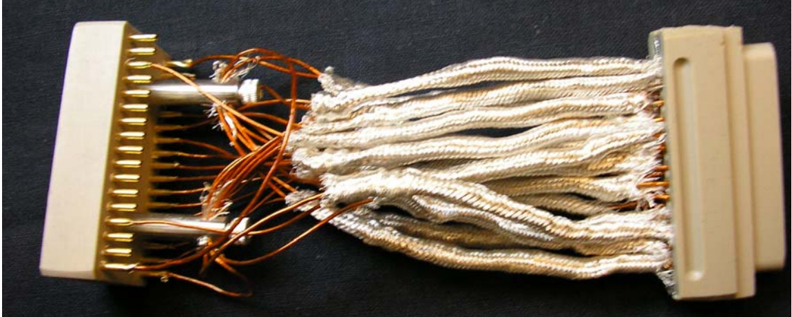
Figure 30. Wiring between Detector and Peek Connector
