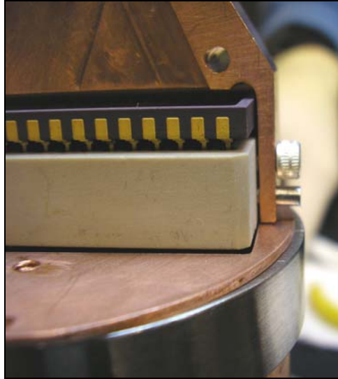
Figure 35. Close-up of Alignment Pin and Screw for PEEK-Aperture Connection
