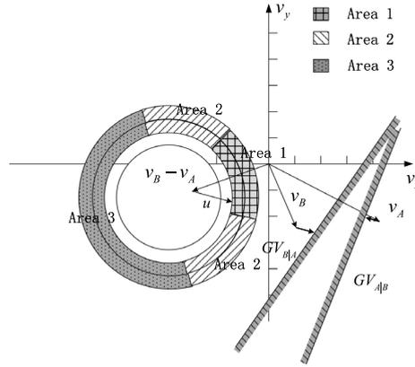
Fig. 4. Grouping velocity constrained area.
