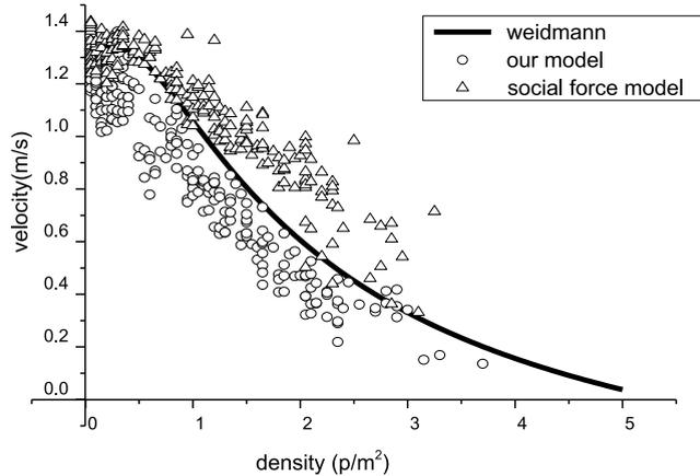
Fig. 11. Density-flow fundamental diagram.
