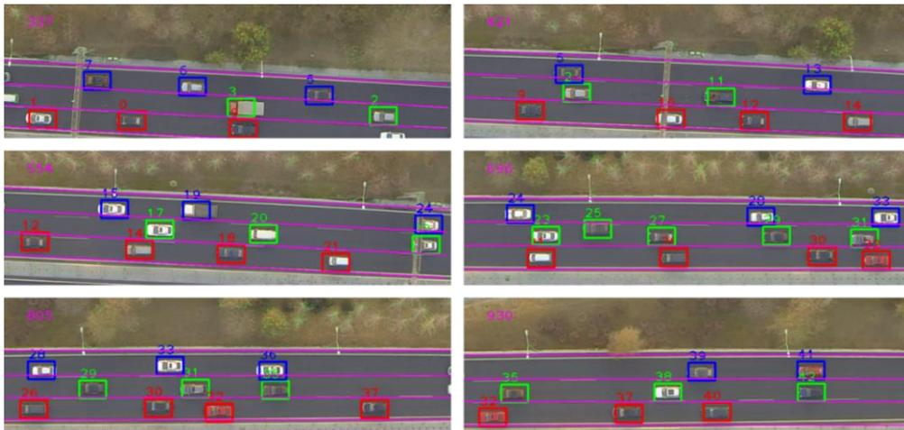
**FIGURE 1 Example frames showing the results of lane detection and multiple vehicle detection/tracking.**
