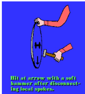
Figure 12: Fixing a flat spot
