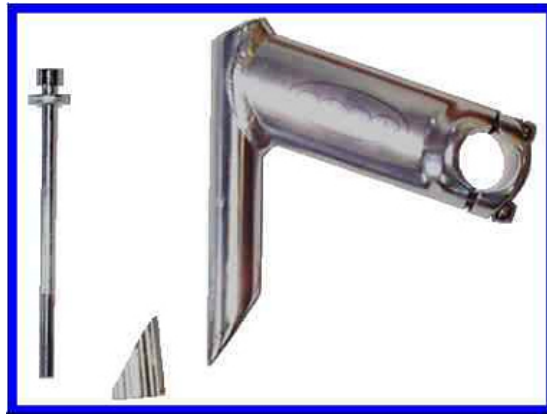
Figure 4: Older style, but still common 'threaded' stem. Long bolt at left goes through stem, pulls wedge tight against inside of steering tube (fork).
