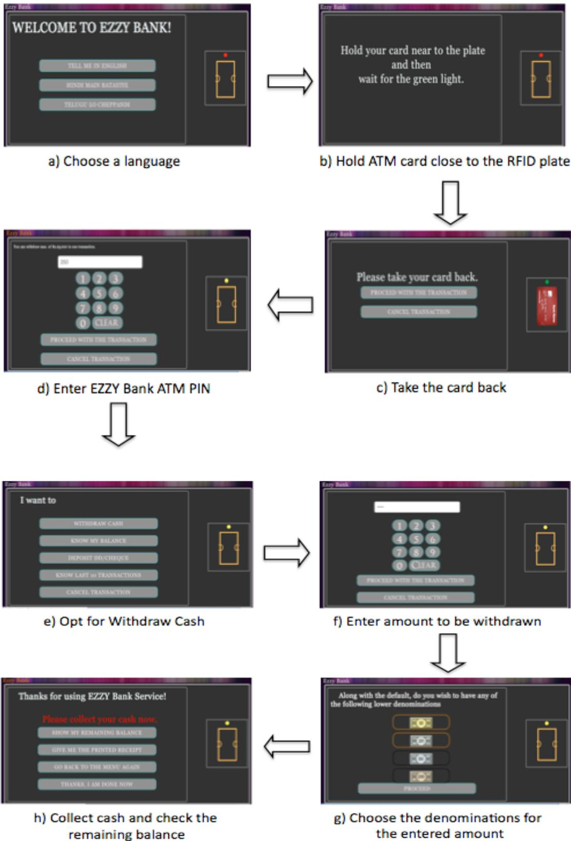
Figure 2: The flow of actions to perform a cash withdrawal operation with the proposed design
