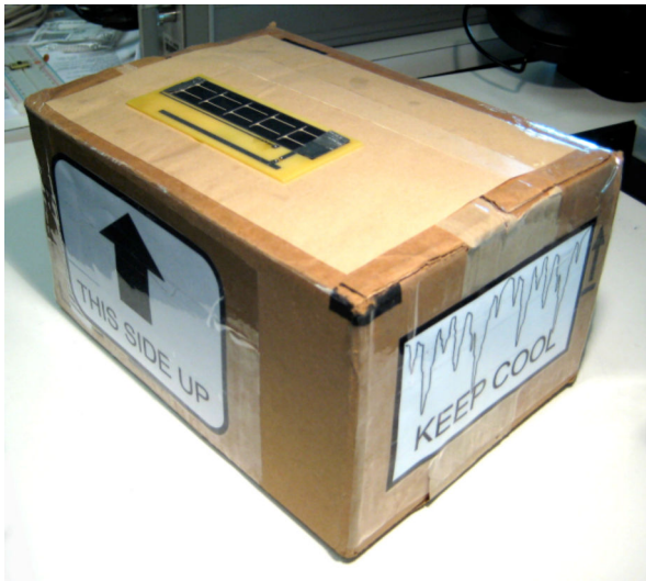
Figure 9. Passive solar antenna-based data logger on a parcel.
